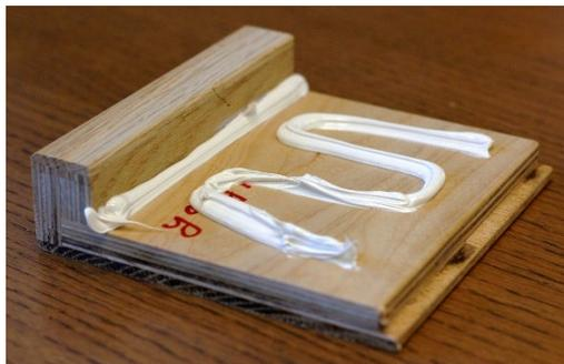
**5/8" Flooring, Single thickness shims pre-applied** – Adhesive installation only recommended. Lay a minimum of 3/8" bead of adhesive in the 90-degree corner located on the back of the bullnose portion of the nosing. Lay an additional 3/8" wavy line of adhesive in between the accommodating foam shims. **Do not place adhesive on the shims.**
