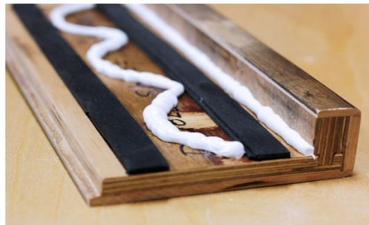
**3/4" Flooring, Double thickness shims pre-applied** – Adhesive installation only recommended. Lay a minimum of 3/8" bead of adhesive in the 90-degree corner located on the back of the bullnose portion of the nosing. Lay an additional 3/8" wavy line of adhesive in between the accommodating foam shims. **Do not place adhesive on the shims.**
