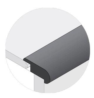
**Application** – The Stair Nose molding combines style and function to create an attractive molding that catches the brunt of floor traffic while enhancing the beauty of a staircase or step. The Stair Nose also provides the proper overhang for a transition from one floor level to the next, such as the step into a sunken living room.
