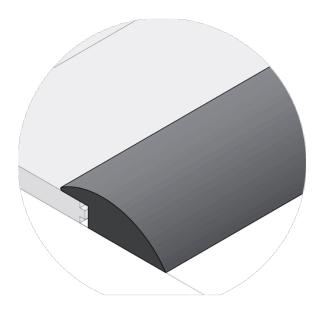
**Application** – Used to join hardwood floors with floors of different heights such as vinyl, ceramic tile or low pile carpeting.
