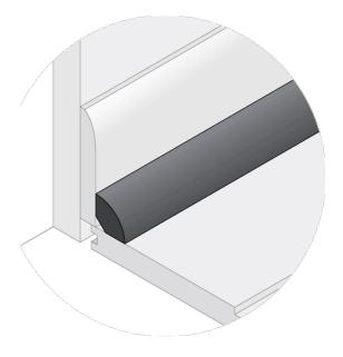
**Application** – The Quarter Round is used in much the same manner as a Wall Base molding to conceal the required expansion space between the wall and the hardwood flooring. It is sometimes used under cabinet toe kicks where a Wall Base won't fit or at the base of a stair to provide a subtle blend between the floor and the wall or vertical surface. Adding the Quarter Round in front of a Wall Base softens the transition and adds a decorative touch.
