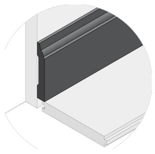
**Application** – Borders the wood floor at the base of the wall to give the room a finished look. This molding helps conceal the required expansion space between the wall and the hardwood flooring. It is also sometimes used under cabinet toe kicks.
