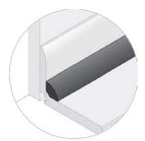
**Base Shoe** – The installation instructions for Base Shoe moldings on a floating floor are the same as a glue down/nail down installation. See the "glue down/nail down" section of this installation guide for instructions on how to install Base Shoe.
