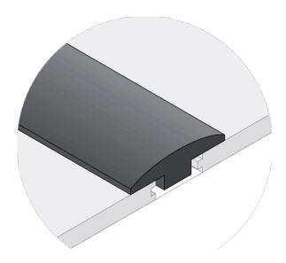
**Application** – Commonly used in doorways to join two wood floors in adjoining rooms. Also recommended when making a transition from a wood floor to another floor that is approximately the same height such as ceramic tile. T-Moldings are also used to provide expansion joints when a floor dimension exceeds 40 feet.
